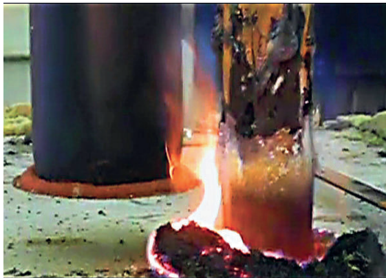
Firestopped Pipe vs Unprotected pipe
